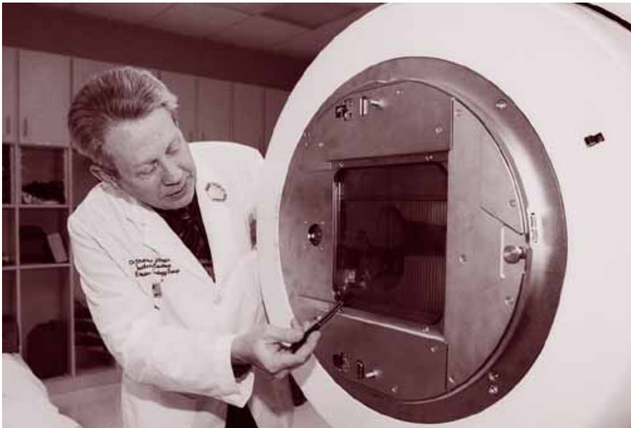
Dr. Sheldon Johnson describes how a state-of-the-art linear accelerator works at the Mary Bird Perkins Cancer Center in Hammond. The new technology uses advanced computer programming that allows adjustments to the intensity of radiation in proportion to tumor thickness and shape. - Photo by Kari Wheeler, Hammond Daily Star.
